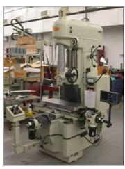
Rebuilt Jig Borer with Digital Readout.
